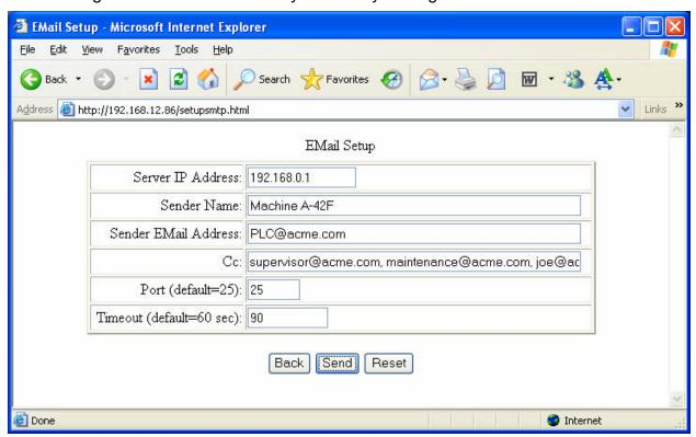
During normal execution, the ECOM100 uses a "working copy" of this data. The data on this page is copied from ROM to the "working copy" in RAM at power-up, and the user can modify any field(s) in the "working copy" using the EMail Configuration (EMLCFG) IBox instruction, allowing for dynamic configuration based on events in the ladder program.
