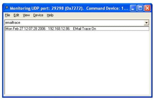
If it reads "EMail Trace **Off**", type in the emailtrace command again to toggle tracing back on.
